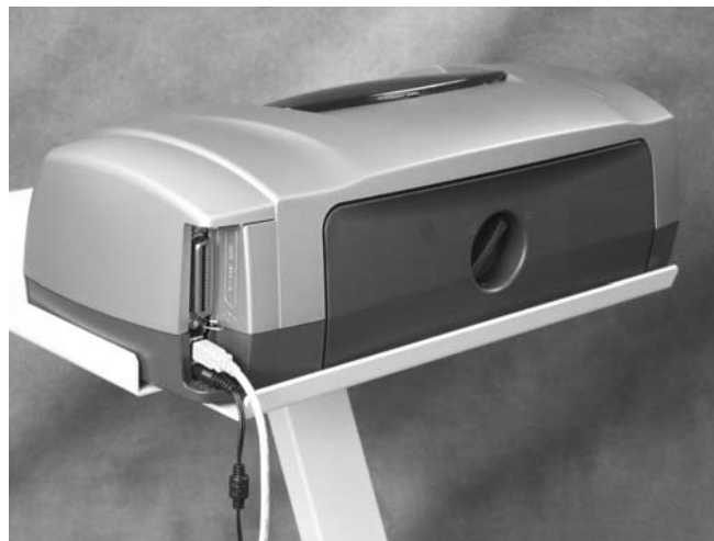
Figure 3.2. Connect the power cable and USB cable to the rear of the printer.
